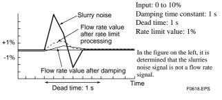
**[J23: Pulsing Flow]** Selection of pulsing flow support In a situation where pulsating flow causes error in the average flow value, due to the application of a plunger pump, this parameter provides functionality whereby calculation is controlled and variations in flow rate are followed.
